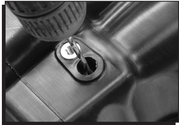
Figure 6 Drilling the MAP Sensor Hole.
