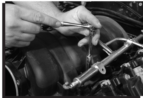
Figure 5 Removing the Intake Retainers.
