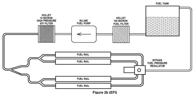
4. Connect the outlets of the regulator to the carburetors.
