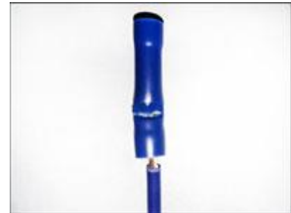
Broken Butt Connectors
