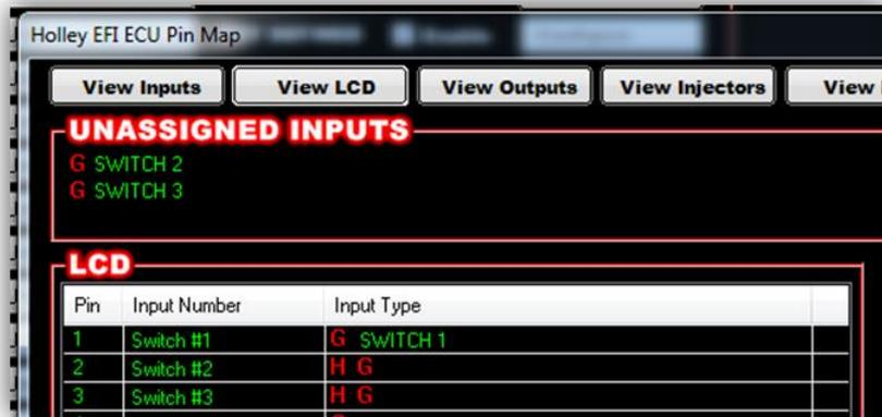
5. Select 'View Outputs' from the 'Pin Map' and drag the outputs to the pin location the device was wired to.
