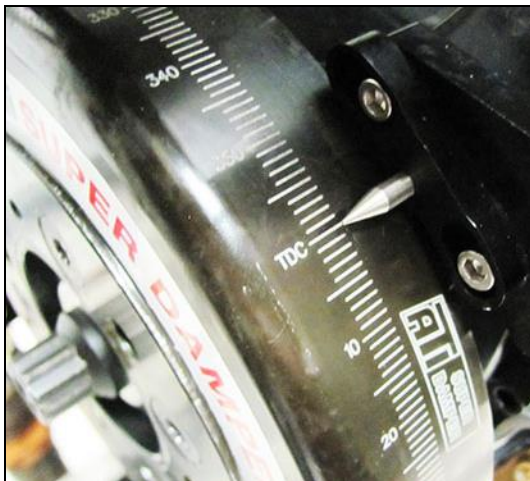
Figure 5: Rotating the Engine to TDC #1
