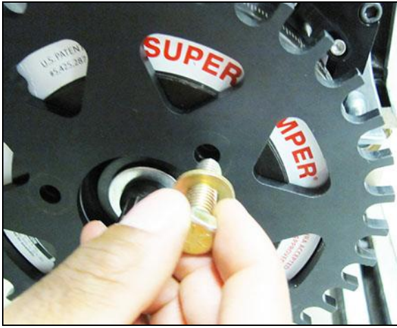
Figure 7: Fastening the Crank Wheel to the Balancer
