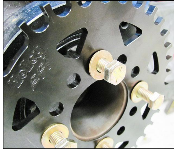
Figure 7: Fastening the Crank Wheel to the Balancer
