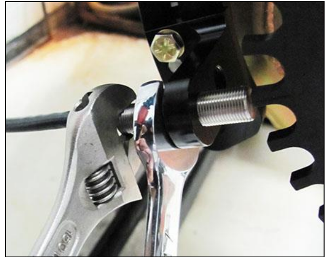
Figure 9: Locking the Sensor Gap
