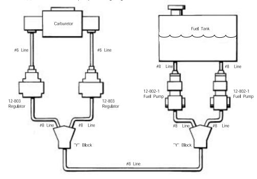
Figure 3 – Two (2) #12-802-1 "blue" pumps feeding single carburetor.
