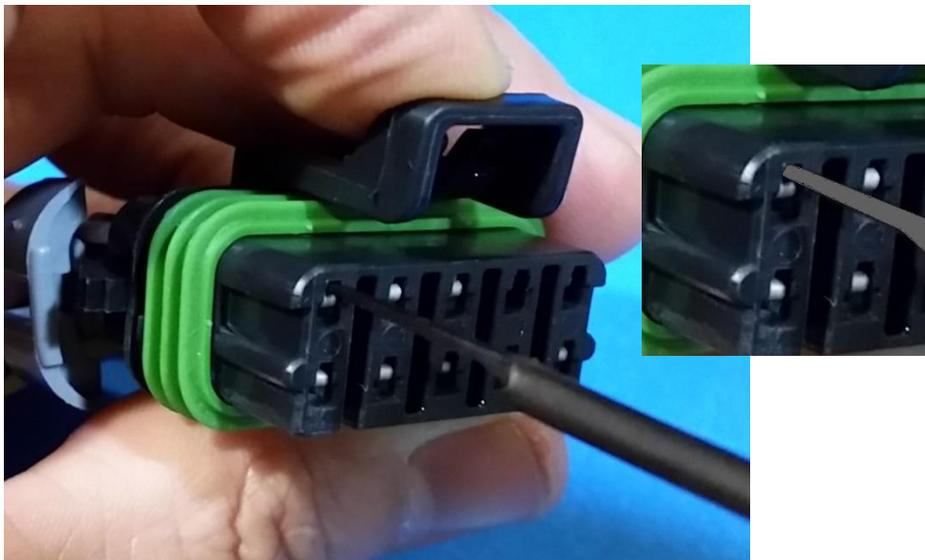
3. After you remove a terminal, replace it with one of the red cavity plugs included in the kit. The Sniper ships with two cavity plugs in the 10-pin connector so you can use these as a reference on how the should be inserted.
