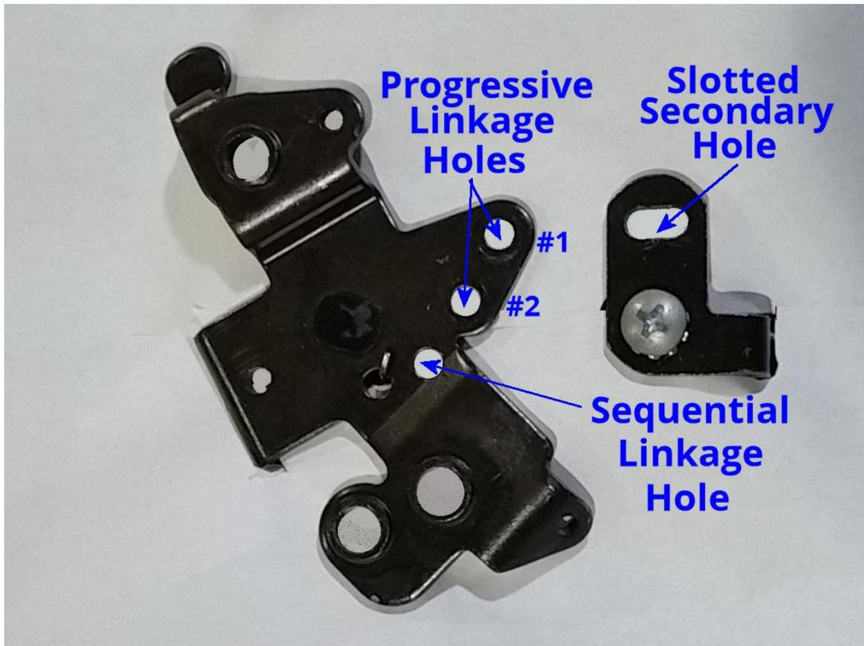
Detailed View of Primary and Secondary Linkage Levers
