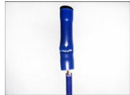
Broken Butt Connectors
