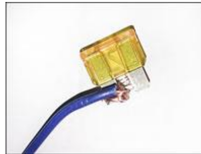
Wire Jammed Into a Fuse
