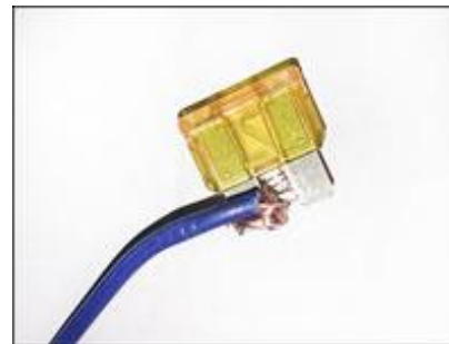
Wire Jammed Into a Fuse
