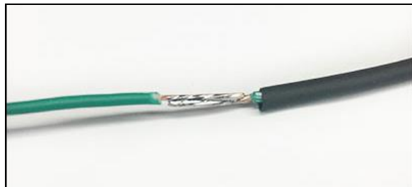
Soldered Connection w/ adhesive heat shrink
